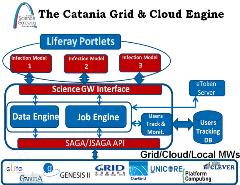
Science gateway layer: This layer consists of the different applications (represented as: infection model 1, model 2, and model 3) that has been ported and deployed on the science gateway.
